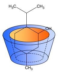
Menthol is an efficient natural cooling agent, with a distinctive odor. Menthol W8 is a commercially available stabilized cyclodextrin inclusion complex with CAVAMAX<sup>®</sup> W8. This formulation provides improved water solubility, and a long lasting cooling effect, but with a low odour.
